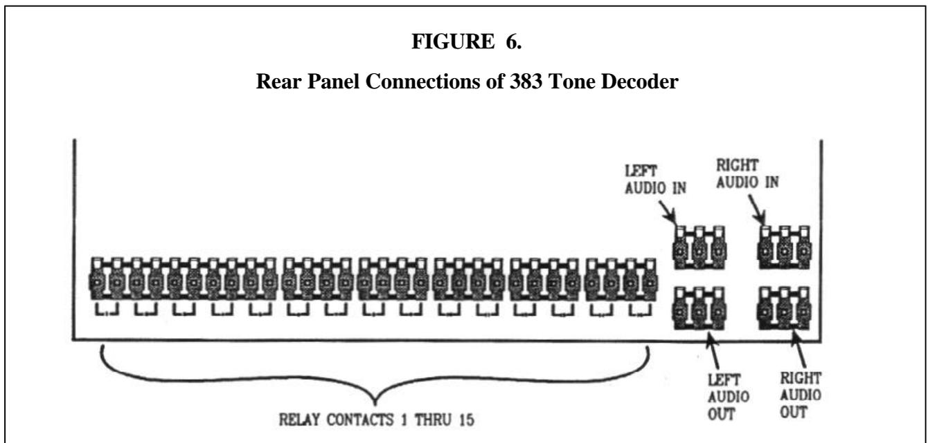
**Control Function Outputs:** (See Figure 6, above for rear panel connections)
